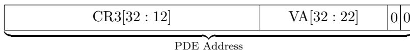
Figure 4.7: Combination of base address in CR3 register with Directory offset in VA to produce the PDE Address
