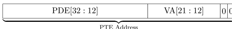
Figure 4.8: Combination of base address in PDE with Page Table offset in VA to produce the PTE Address
